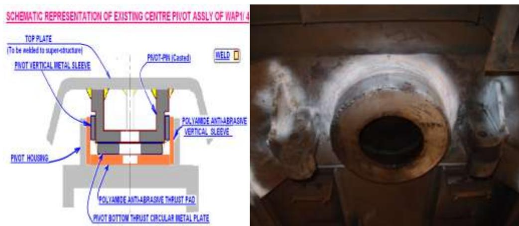
Fig. 1 schematic of pivot pin welding Fig. 2 pivot pin welding with mounting plate
