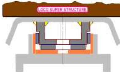
Fig. 4 Schematic representation of center pivot assembly of WAP 4
