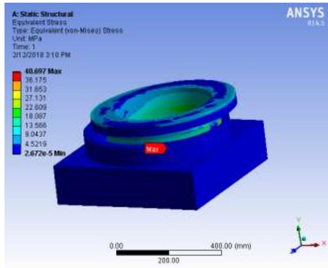
Fig. FEA Analysis for Pivot Pin with collar
