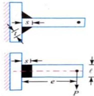
Fig. 3 Eccentrically Loaded Welded Joints
